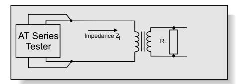
The return loss is a measure of the impedance mismatch between the transformer and a transmission line.
