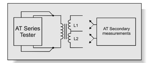
The inductance of a winding is determined by the number of turns and the construction and dimension of the core materials; it may also vary with test conditions such as voltage and frequency. See the LS and LP tests
