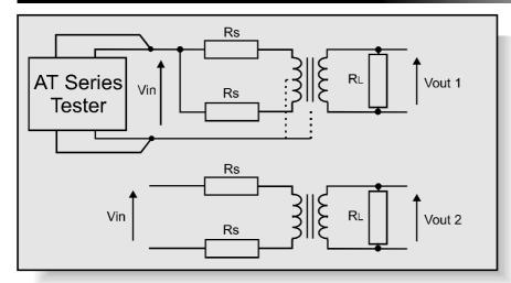
Longitudinal balance is a measure of the common mode rejection ratio (CMRR) of a transformer. That is, the ability of the transformer to reject unwanted noise signals that are common to both input terminals with respect to a common point.
