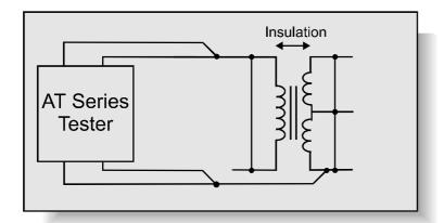
Transformer windings are often insulated from each other and from the core by insulating tape, enamel on the wire or by plastic moulding on the bobbin.
