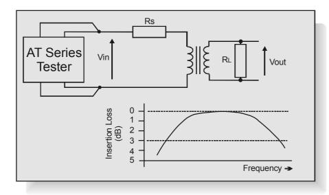
Frequency response is a measure of how the power lost by a transformer (inserted into an impedance matched transmission system) varies with frequency.
