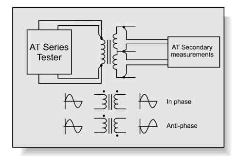
Applying an ac voltage to the primary of the transformer will produce an ac voltage in the secondary. Turns ratio describes the voltage ratio of the measured voltages from one winding and another.
