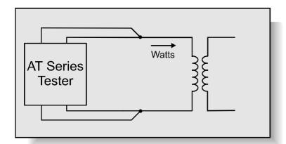
At no load, and with its secondaries open circuited, a transformer will still draw current and consume power as described in the WATT test.
