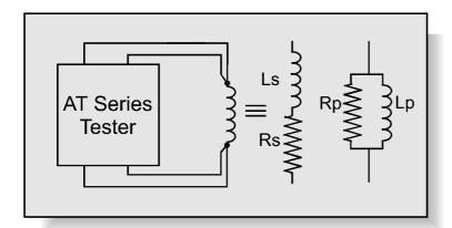
Inductance is the electrical parameter that is commonly used to check that a high frequency transformer has been constructed according to its design and that it will operate properly in use.
