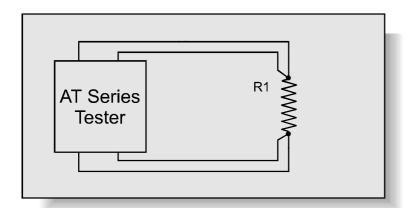
R1 represents the resistance of the copper wire used to wind the transformer. When current flows in the winding, the resistance causes losses in the winding (I²R losses), which cause undesirable heating within the transformer.
