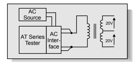
Open circuit voltage is the voltage appearing across a secondary winding when the primary is energized at a specified voltage and frequency.
