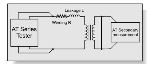
Due to imperfections in the coupling between windings, a short-circuited transformer acts as if there is inductive impedance in series with the winding.
