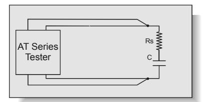
'Dissipation factor' or 'tanô' is most often used as a measurement of the losses in a capacitor. It is analogous to 'Q' for an inductor.
