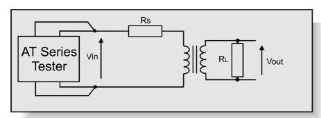
The insertion loss is a measure of the power lost by a transformer relative to the maximum theoretical power that the transformer could transmit to a given load.
