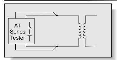
The wire used to wind a transformer may contain defects in its insulation. For example, scratches in the enamel of copper winding wire. This test may be used to highlight insulation defects between adjacent turns in a winding as opposed to insulation defects between windings.
