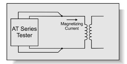
Magnetizing current is the term used to denote the total current that flows into the primary of a transformer when the transformer is energized at a specific voltage and frequency, with the secondaries open circuited.
