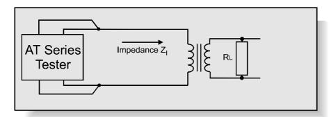
The impedance of a transformer is usually complex, that is it consists of real (resistive) and inductive or capacitive (imaginary) parts. The total impedance at a specified frequency is the vector sum of these parts.
