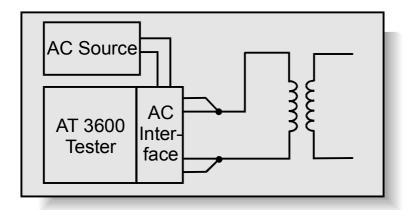
At no load, with the secondaries opencircuited, a transformer will still draw current and consume power. The current is typically only a few percent of the normal full-load current, and the I<sup>2</sup>R copper loss is thus negligible. The measured power is then the power dissipated by eddy current and hysteresis effects in the core and is known as the core loss.
