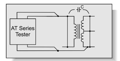
Capacitance occurs in transformers due to the physical proximity of, and electrostatic coupling between, different turns of wire.
