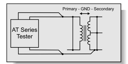
Transformers may be used to provide isolation between dangerous line input voltages and safe low voltage outputs.
