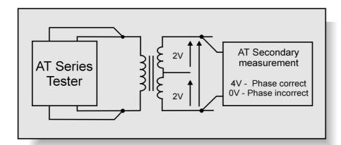
Open circuit voltage is the voltage appearing across a secondary winding when the primary is energized at a specified voltage and frequency, with the secondary at no load.
