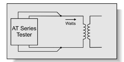
At no load, with the secondaries open circuited, a transformer will still draw current and consume power. The current is typically only a few percent of the normal full-load current, and the I<sup>2</sup>R copper loss is thus negligible. The measured power is then the power dissipated by eddy current and hysteresis effects in the core and is known as the core loss.
