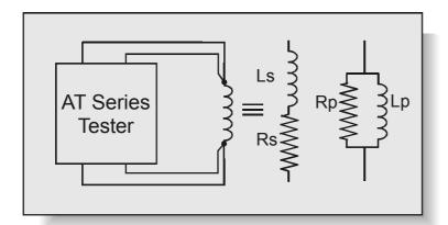
Inductance is the electrical parameter that is commonly used to check that a high frequency transformer has been constructed according to its design and that it will operate properly in use. As well as operating with ac signals, some transformers and chokes are designed to operate with a dc bias current flowing in a
