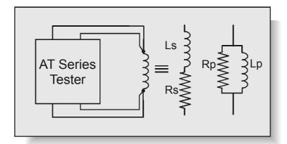
The equivalent ac resistance of a winding may be different to that measured at dc. The resistive part of the complex winding impedance will vary with frequency due to skin and proximity effects.
