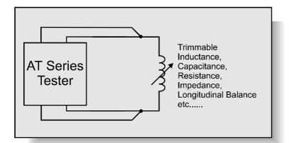
In critical applications, or where the best transformer performance is desired, it may be necessary to trim a particular component parameter to be within desired limits.
