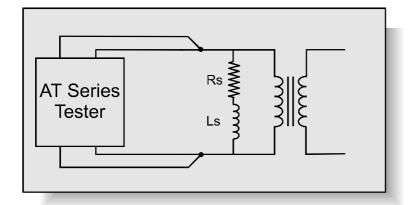
When a transformer is energized, the changing magnetic field in the core causes two types of losses:- hysteresis losses and eddy current losses. The total of these losses can be represented on the equivalent circuit of a transformer by a resistance associated with the inductance of the winding.
