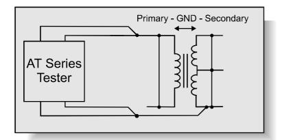
Transformers may be used to provide isolation between dangerous line input voltages and safe low voltage outputs. The transformers may be separate line frequency transformers or power or control transformers inside power supplies and similar equipment.
