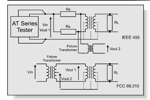
Longitudinal balance is a measure of the common mode rejection ratio (CMRR) of a transformer. That is, the ability of the transformer to reject unwanted noise signals that are common to both input terminals with respect to a common point.
