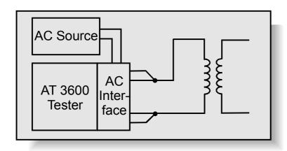
At no load and with its secondaries open circuited, a transformer will still draw current and consume power as described in the WATT test.
