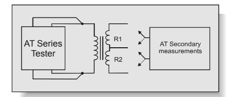
R1 and R2 represent the resistance of the copper wire used to wind the transformer. When current flows in the windings, the resistance causes losses in the windings (I²R losses), which cause undesirable heating within the transformer.
