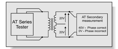
Open Circuit Voltage (VOC) is the voltage appearing across a secondary winding when the primary is energized at a specified voltage and frequency, with the secondary at no load.
